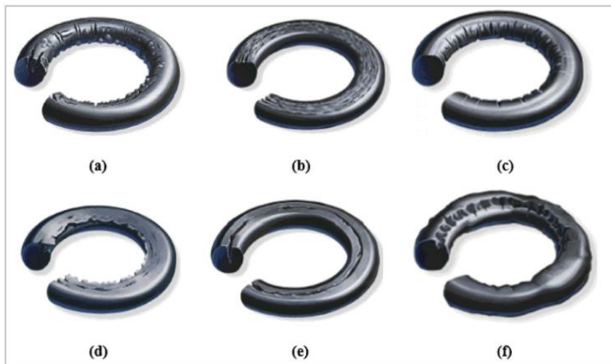
Figure 6. Failures in elastomer O-ring: (a) explosive decompression, (b) abrasion friction, (c) thermal degradation, (d) extrusion, (e) compression set, (f) chemical degradation.
